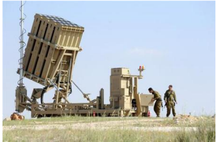
The Iron Dome, also known as "Iron Cap" is a mobile all-weather air defense system developed by Rafael Advanced Defense Systems. It is a missile system designed to intercept and destroy short-range rockets and artillery shells fired from distances of 4 to 70 kilometers away and whose trajectory would take them to a populated area.
